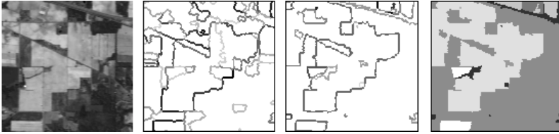
Fig. 3. Satellite image results. From left to right, original image (band 120), results using the band selection, results using the same selected bands and illumination invariants and the final segmentation represented with random colors.
